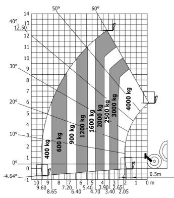
Machine on lowered stabilisers with forks Metric
